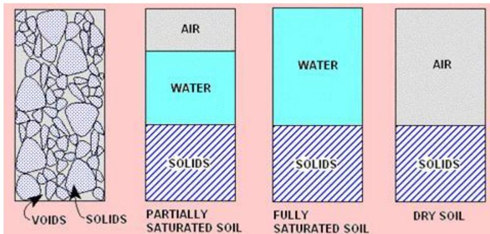
For the purpose of engineering analysis and design, it is necessary to express relations between the weights and the volumes of the three phases.
