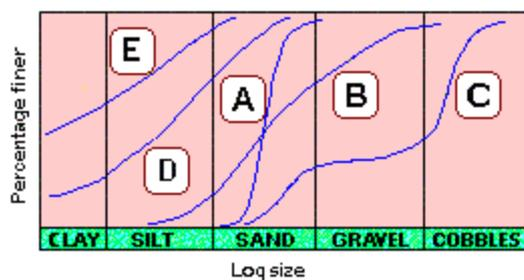
**Curve A** - a poorly-graded medium SAND
